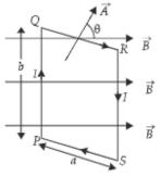
Force on side *PQ* or *RS* of loop is  $F = IbB \sin 90^\circ = Ib B$  and perpendicular distance between two non-collinear forces is  $r_{\perp} = a \sin \theta$
