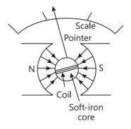
Its working is based on the fact that when a current carrying coil is placed in a magnetic field, it experiences a torque. This torque tends to rotate the coil about its axis of suspension in such a way that the magnetic flux passing through the coil is maximum.
